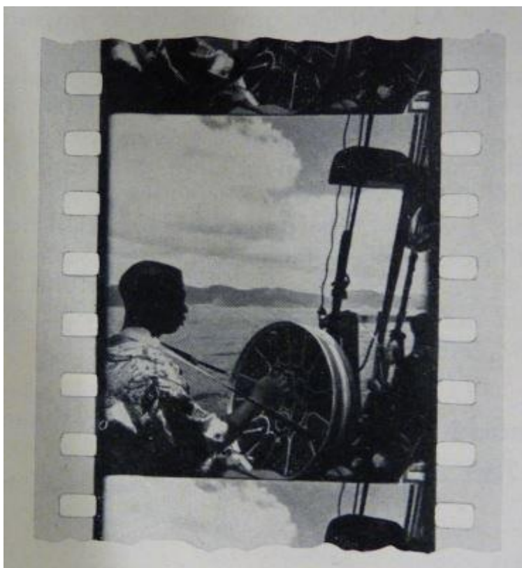
Left: an original cinematic image from the left panel of Windjammer . It is from a film scene that can be seen shortly after the film's intermission. It has a height of 27.9 mm with respectively 6 perforation holes on both sides. Windjammer was filmed and projected at 26 fps (frames per second). 44,6 metres of film run through the projector every minute.
