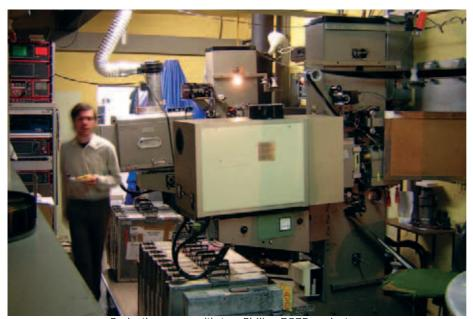
Projection room with two Philips DP75 projectors. Note 70mm transportation boxes under lamp house.
