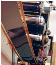
Close up of 70mm film with magnetic sound – brown oxide strips on edge of film.
