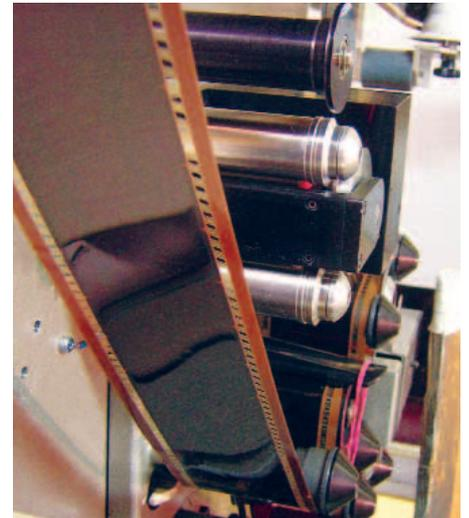
*Close up of 70mm film with magnetic sound – brown oxide strips on edge of film.*
