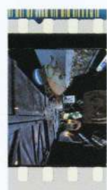
Conventional 35mm, 24fps film (actual size) with optical soundtrack. The strip shows the actual amount of frames photographed in just under 1/2 second. In 35mm film each frame is photographed at 1/24th of a second, and then projected twice. Frames are spaced against Showscan® 70mm, 60fps which shows how little information is actually recorded by 24fps photography. The white gaps clearly show how much action, emotion, and motion put before the camera is "missing" with the standard process.
