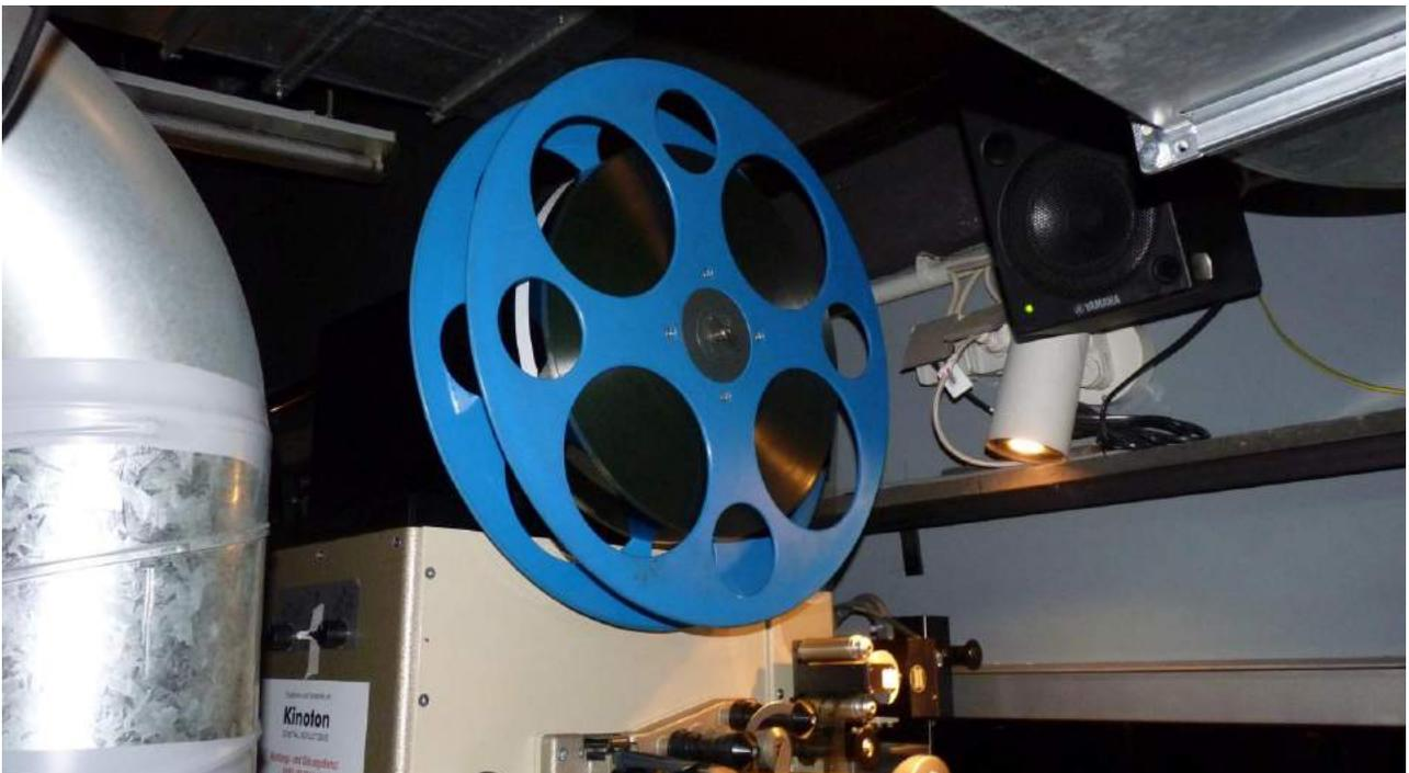
**The 21-minute 70mm silent film "EQUINOX" [70mm (5-perforation holes), color, AR 1:2.1] in the film reel of a Kinoton FP75 E projector. The company "KINOTON Digital Solutions" (also based in Berlin) is responsible for maintenance work on the device.**
